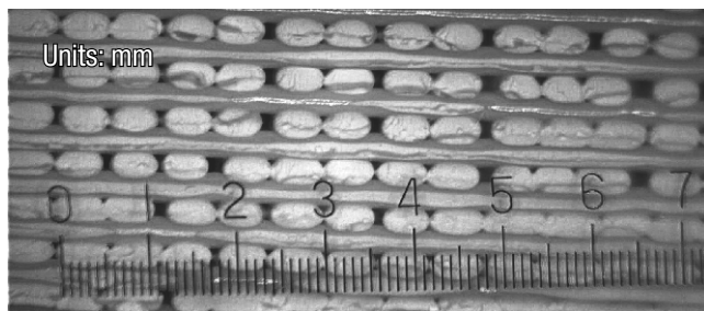
Figure 17: The internal structure of a ‘solid’ wall made with an FDM 3D printer has gaps on the order of 200 μm. This irregular structure likely causes THz radiation to scatter inside.
